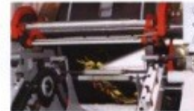
Bottom Forming Drum: Center Grippers, Clamps, and Drum Fingers are Spider Mounted for ease of changeover.
